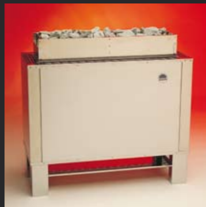
34.G Professional Free-standing heater Free-standing heater for the commercial sauna. Triple shell design in two sizes: 15.0 - 21.0 kW as well as 24.0 - 36.0 kW. Inside and outside shell completely made from high grade steel. Large stone basket. Radiated heat and convection due to the appropriate amount of stones.
