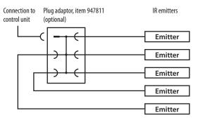
By 750 W radiators max. 4 units (3500 W) possible by 16 A capable connection line. Plug adaptor 947811 - optional.
