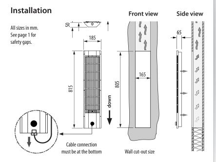
**Risk of fire!** Make sure to provide sufficient air circulation behind and above the heater. The space above the raditor must not be blocked, so that the warm air may rise freely. Do not install in the ceiling!
