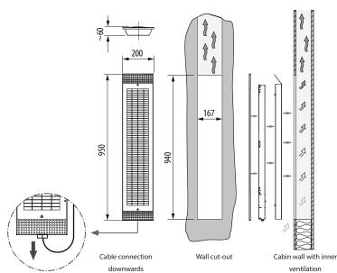
Vertical installation into the cabin wall
