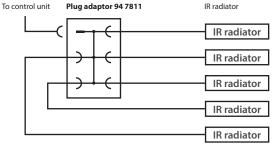
By 750 W radiator max. 4 units (3500 W) possible by 16 A capable connection line.
