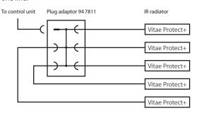
By 750 W radiator max. 4 units (3500 W) possible by 16 A capable
