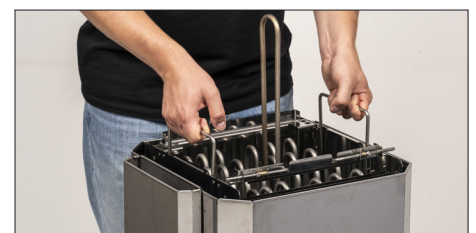
Morpheus PRO : Modular construction with removable rock store and heating block significantly reduces service and maintenance time.
