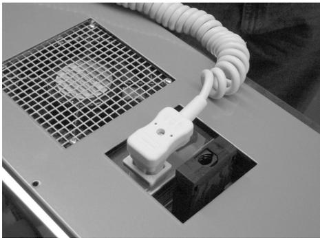
Connect the power cord leads to 230 V.
