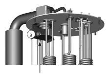
Check all screws for tightness before commissioning. Connect the steam pipe (b) to the bottom of the housing. Place the flexible water pipe on the water inlet valve and fix it with the hose clamps (c). Attach the descaling hose (d) to the connection nipple for the descaler.
