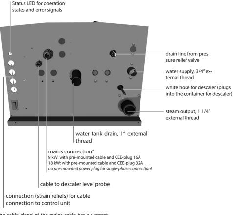
\* The cable gland of the mains cable has a warrant seal. Make sure not damage the seal. Warranty void by damaged or removed seal.
