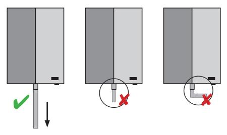
Example of a correctly and incorrectly installed drain line for rinsing
