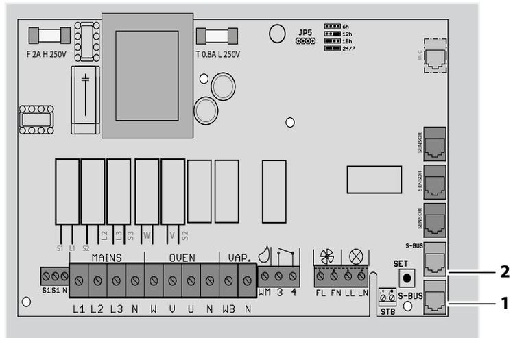
Jacks – relay box for steam generator/relay box for sauna cabin and IR cabin
