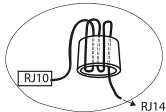
The ferrite ring for jack #1 is included in the scope of delivery for each control panel and add-on module.
