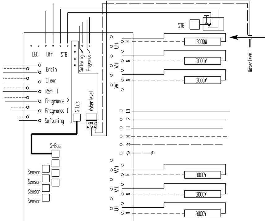
Diagram of circuit board (18 kW example) – connection U1 for colour-coded heating coil
