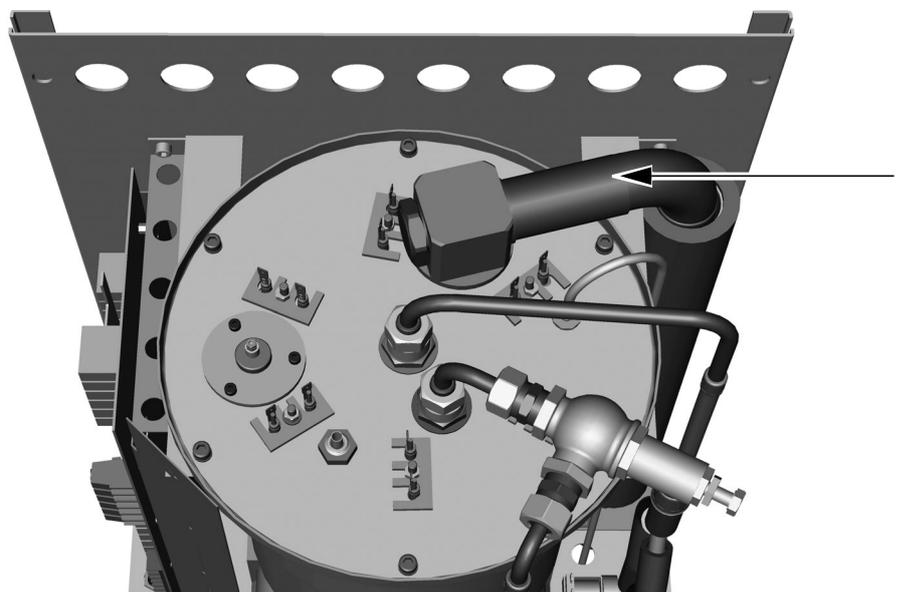
Lay the steam pipe so it descends towards the steam outlet without any sharp 90° bends.
