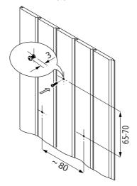
Horizontal distance between drill holes: 80 mm
