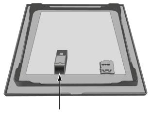
① The control line's RJ10 plug is inserted into the circuit board on the control panel. The RJ14 plug is inserted into the relay box.
