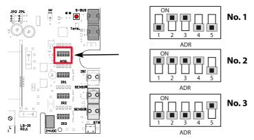
① The relay box is set to address no. 1 by default. As a rule, this setting must not be changed.
