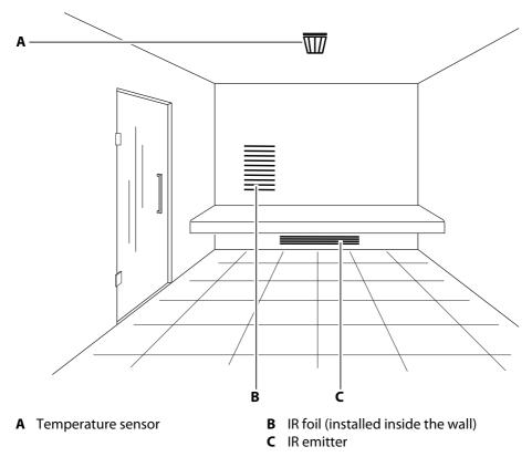
The position and number of IR emitters and foils (IR emitters) can vary depending on the design of the cabin.
