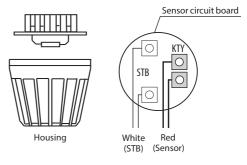
5. Lead the sensor cables through the right cable intake into the control unit. Install the sensor cables inside the control unit as shown in Fig. 11.
