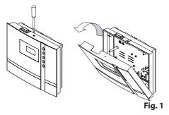
Remove the control device cover. In order to do this loosen the screw at the top of the housing and pull the housing top upward while swivelling (Fig. 1).
