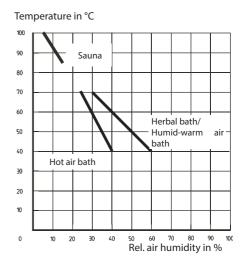
The humidity intensity shown in the display corresponds to the time-proportional vaporizer setting. Therefore the relative air humidity is <u>not</u> pre-selected or shown in the display, instead the activation frequency of the vaporizer is shown as a percentage. This is explained in the diagram.
