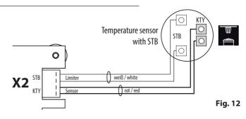
6. After completed installation and before commissioning of the control unit the line for overheating protection fuse must be checked for proper functionality. For this disconnect one of the white cable wires at X2 connector. The respective error message appears in the display. Re-connect the wire.
