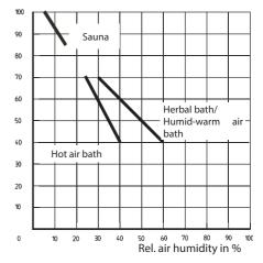
The humidity intensity shown in the display corresponds to the time-proportional vaporizer setting. Therefore the relative air humidity is <u>not</u> pre-selected or shown in the display, instead the activation frequency of the vaporizer is shown as a percentage. This is explained in the diagram.
