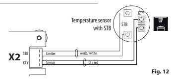
6. After completed installation and before commissioning of the control unit the line for overheating protection fuse must be checked for proper functionality. For this disconnect one of the white cable wires at X2 connector. The respective error message appears in the display. Re-connect the wire.
