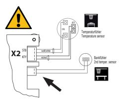
If the sensor is connected correctly, the control unit shall automatically recognise it once the mains voltage has been switched on again.
