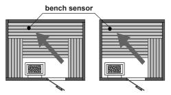
The bench sensor is connected with a 2-core silicone cable from the sensor pcb to the terminals on the right-hand side of the main board of the sauna controller (X2), as shown below.
