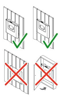
Proper and improper mounting of the control unit
