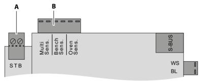
**A** Terminal plug for safety temper- **B** Sensor for safety temperature limiter ature limiter
