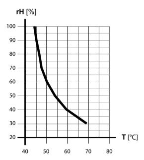
★ Characteristics curve for temperature/humidity
