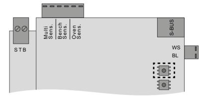
Set the jog dial with the screwdriver as supplied in the scope of delivery.
