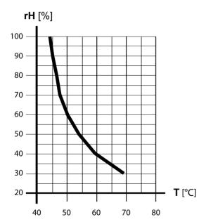
All values that lie below or on the characteristic curve can be set and used. When setting a parameter, e.g. temperature, the setting for the other parameter (humidity) is automatically adjusted.
