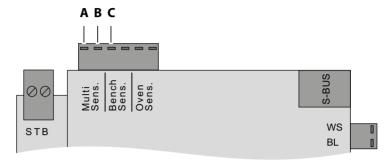
4 Plug the terminal plug into the circuit board again as assigned.
