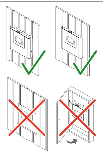
Proper and improper mounting of the control unit
