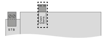
**a)** Connect the cable for the safety temperature limiter from the heater sensor to the 2 **STB** terminals on the lower main circuit board.
