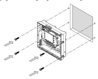
You can connect the lines after mounting the housing. See
