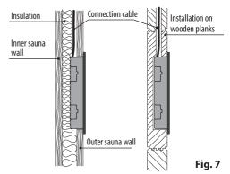
Use the supplied 5 m connection cable with RJ10 plug (control panel side) and RJ14 plug (relay box side).
