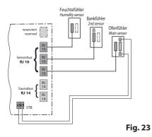
With correct connection, the sensor will be automatically detected and configured. The display will show the following symbol during start-up.
