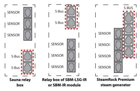
Ercuit board sections for S-Bus jacks
