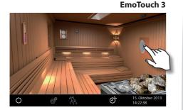
To switch on the sound, brief touch the loudspeaker (EmoTouch). Touching for a longer period opens up the sound settings.
